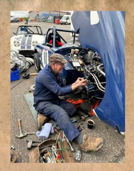
The paddock was busy with through the weekend with repairs and adjustments. John Hughes had a failure in Race 1 with o/s front axle bearing which had welded itself to the stub axle. Richard Perry came to the rescue with a replacement which the Hughes talented spanner man Ian Blaine(see above) fixed for second race.
